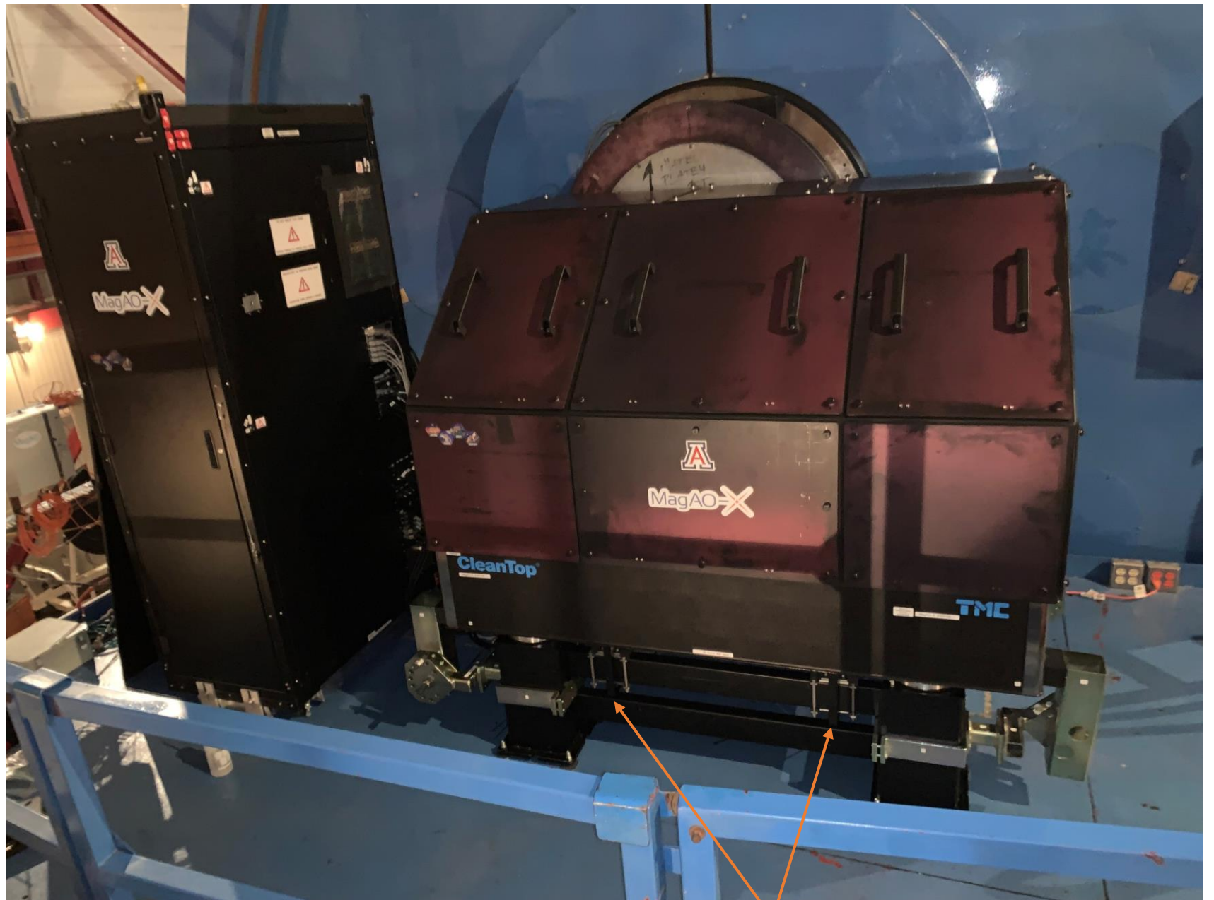
Installed earthquake bars
