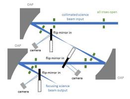
Figure 6: Flip mirror method: flip each flip mirror into the beam in succession down the beam path (with the irises fully open). The reflected beam, both collimated and the PSF, will give tip/tilt error information for the preceding OAP, and the PSF will give higher precision error information for the preceding OAP.
