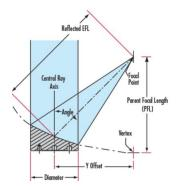
Figure 1: OAP diagram demonstrating the ability to focus an incoming collimated beam while deviating the beam off-axis at a designed reflection angle.
