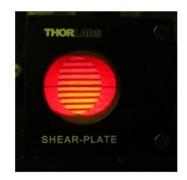
Figure 2: Shear plate interferometer showing straight line fringes indicating the light reflecting off of the OAP is collimated and free of aberrations.(1)
