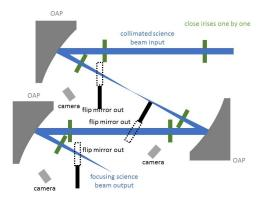
Figure 3: Iris method: close down each iris individually in succession down the beam path (with the flip mirrors out of the beam). Misalignment on the iris will give tip/tilt misalignment information for the preceding OAP.
