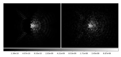
Figure 7: MagAO-X F/69 Science plane PSFs with vAPP coronagraph implemented, for unaberrated (left) and aberrated (right) systems
