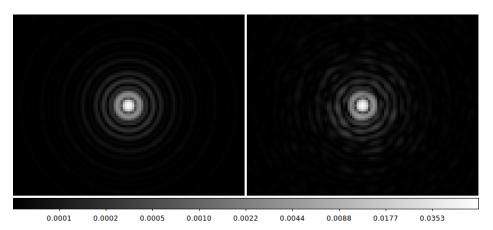
Figure 5: MagAO-X F/69 PSFs for unaberrated (left) and aberrated (right) systems
