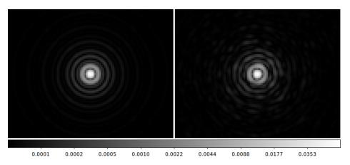
Figure 6: MagAO-X F/69 Science plane PSFs for unaberrated (left) and aberrated (right) systems
