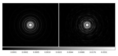
Figure 3: MagAO-X F/16 PSFs for unaberrated (left) and aberrated (right) systems
