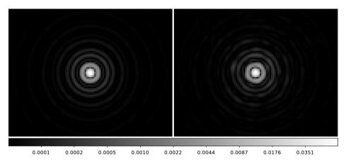
Figure 2: MagAO-X F/11 PSFs for unaberrated (left) and aberrated (right) systems
