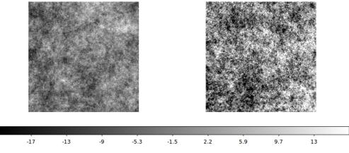
Figure 1: Sample MagAO-X optical surfaces used in POPPY (left: F-0 flat mirror; right: O-0 OAP mirror)
