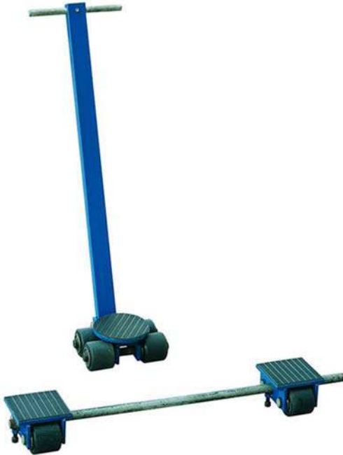
Figure 2.4-5: Industrial moving dolly. It is three point support that eliminates the possibility of a skate to slip out due to uneven loading when traversing uneven and discontinuous flooring. Wide rollers prevent wheel from getting stuck. Model shown has a 6 ton capacity.
