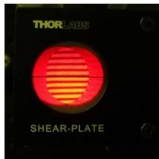
Figure 2: Shear plate interferometer showing straight line fringes indicating the light reflecting off of the OAP is collimated and free of aberrations.(1)
