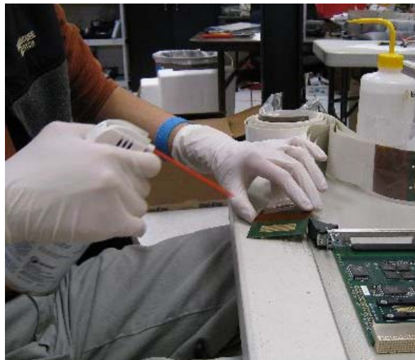
Figure 7. Blow dry both gold-covered connections with an air duster.
