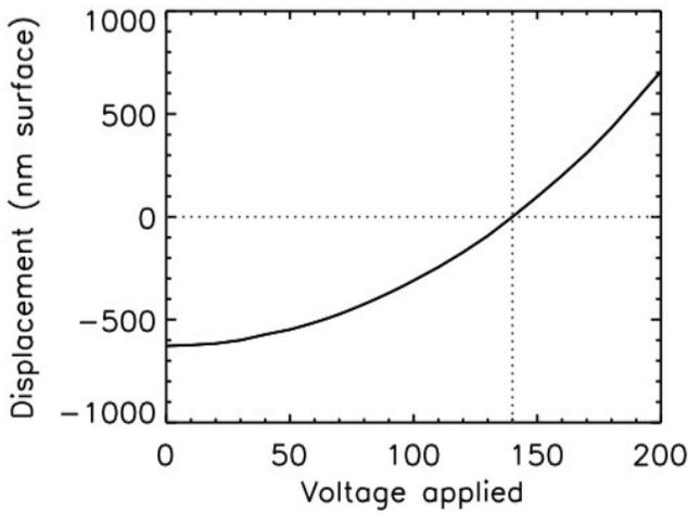
Figure 1: Displacement vs. applied voltage, 1 actuator (Villages MEMS).
