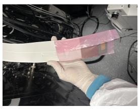
4. Gently lower the bagged ribbon cable to hang down, avoiding kinks. It should not *reach* the floor, but don't let it touch the floor in any case.
