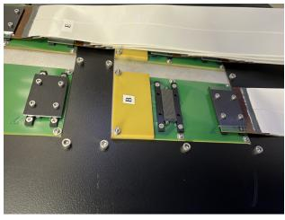
If a pin sticks, very carefully pull it out using needle nose pliers. Do not drop it. Insert it back into the removable connector in the same orientation.
