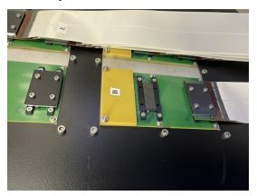
3. Set plate aside, have assistant bag the end of the ribbon cable with an ESD bag. Fold the excess ESD bag over to make it approximately the right width, and use tape to secure ESD bag to itself and to the ribbon cable.
