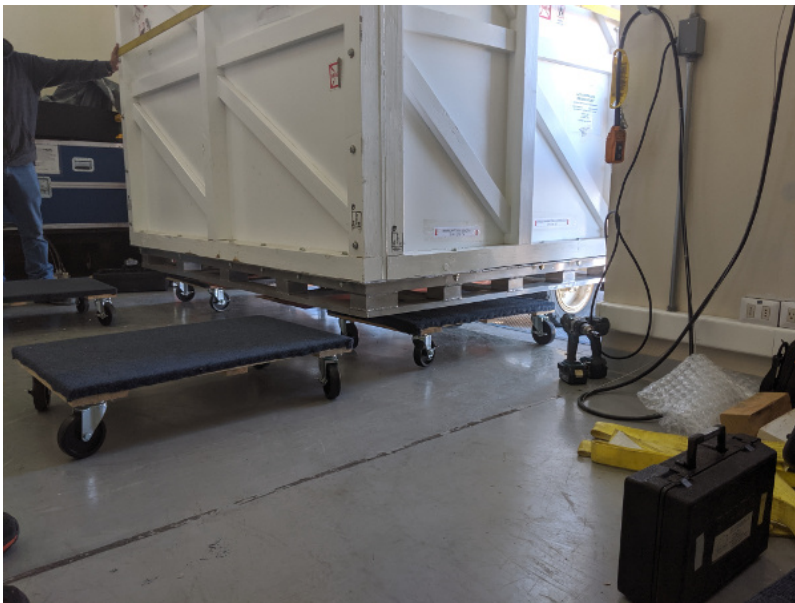
The instrument box being set down on dollies with the fork lift. Note the placement and orientation of the dollies.
