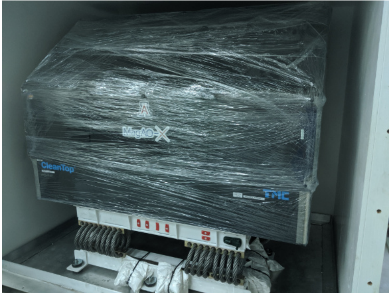
MagAO-X on the shipping frame inside the box.
