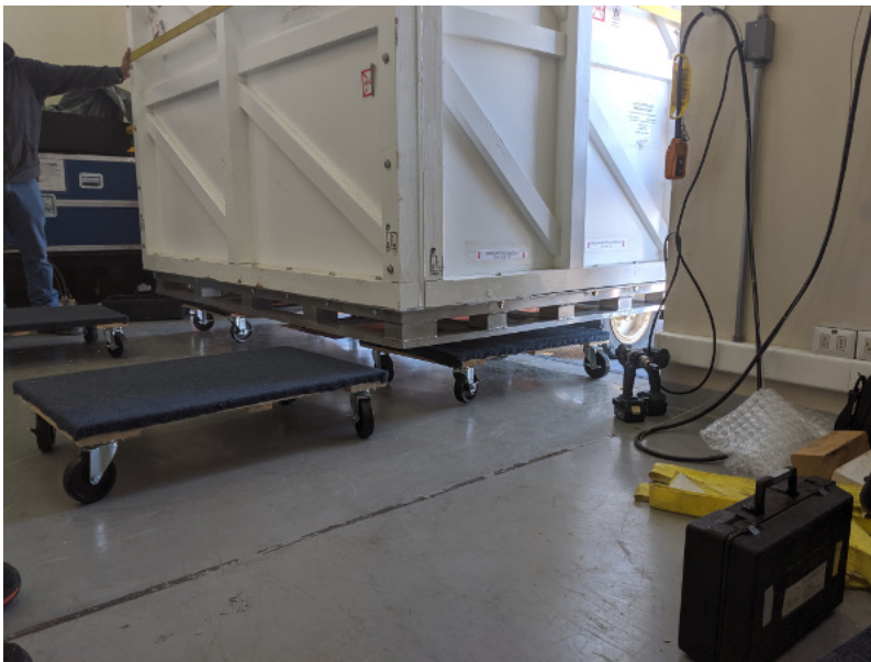
The instrument box being set down on dollies with the fork lift. Note the placement and orientation of the dollies.
