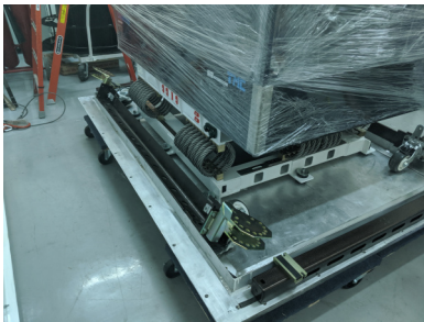
The cart is assembled on the pallet around the instrument. This shows it in progress.
