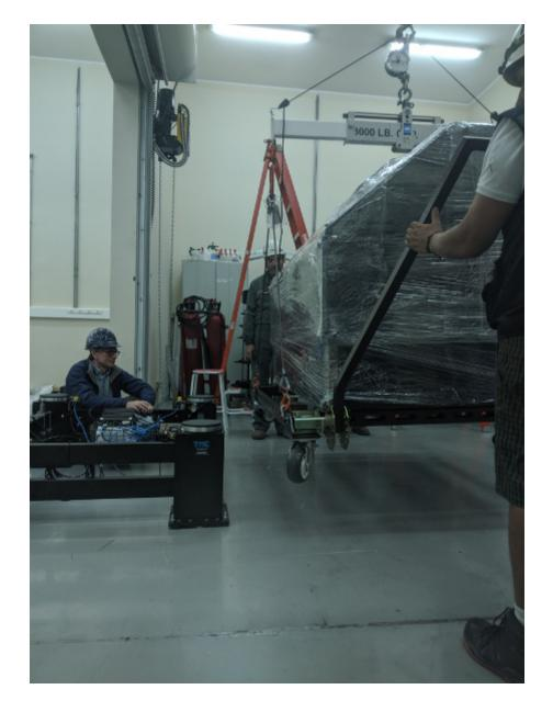
The cart and instrument ready to be set down on the wheels, with legs out of the way.
