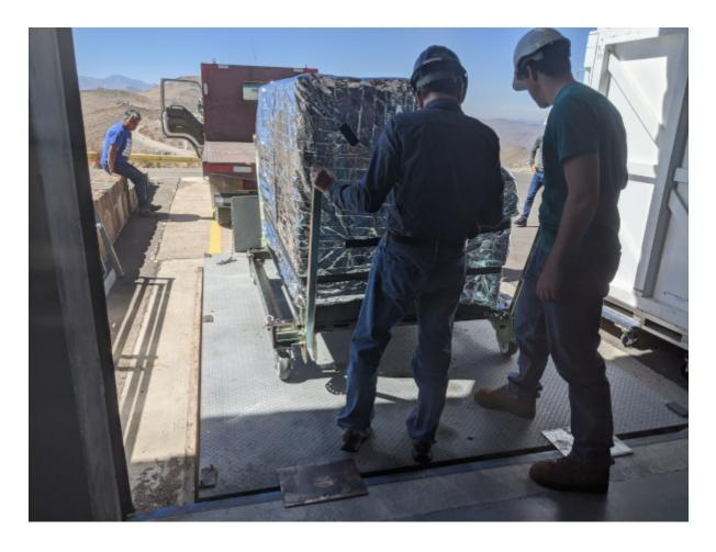
MagAO-X moved onto the pentalift. Note the metal plates across the gap.
