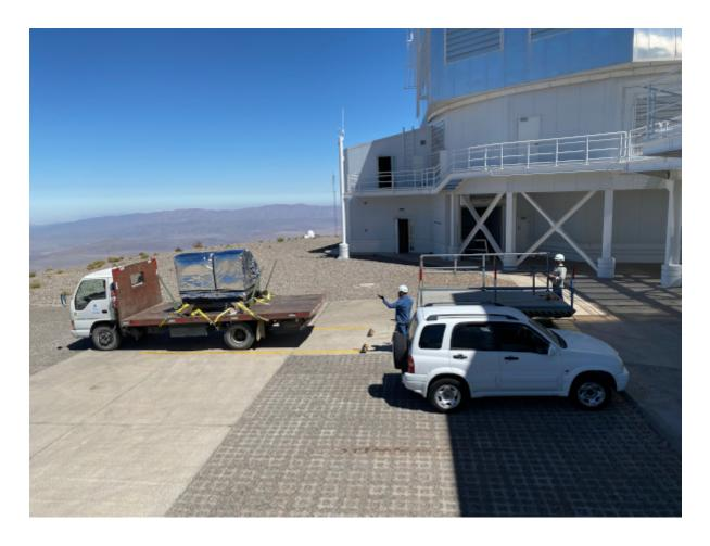
MagAO-X will be unloaded at the telescope using the lift gate, adjusted for slow operation as it is for the ASM.
