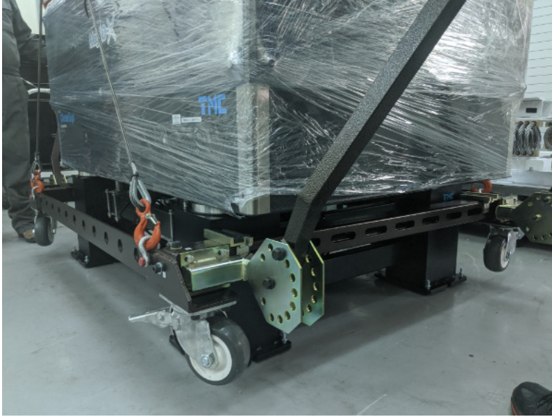
The cart being lifted to the bottom of the table. Note the direction of the hooks.
