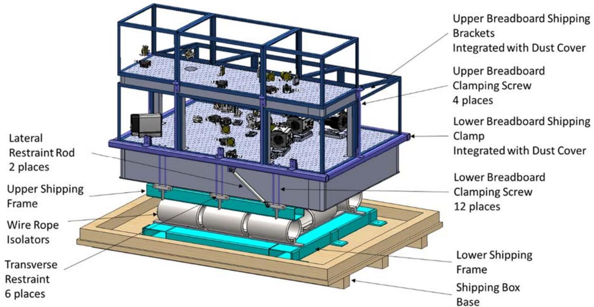
Figure 2.4-3: Optical table crate design details.
