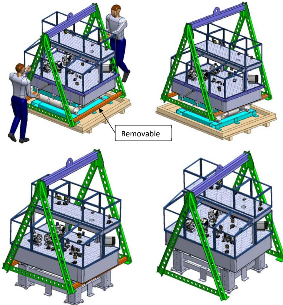
**Figure 2.4-4:** Optical table lifting frame. Top-left and top-right view shows the configuration when lifting the table out of the crate. Bottom-left and bottom-right views shows the configuration when lowering the table onto the legs. Red bars are removed prior to lowering upper frame onto and off of table.
