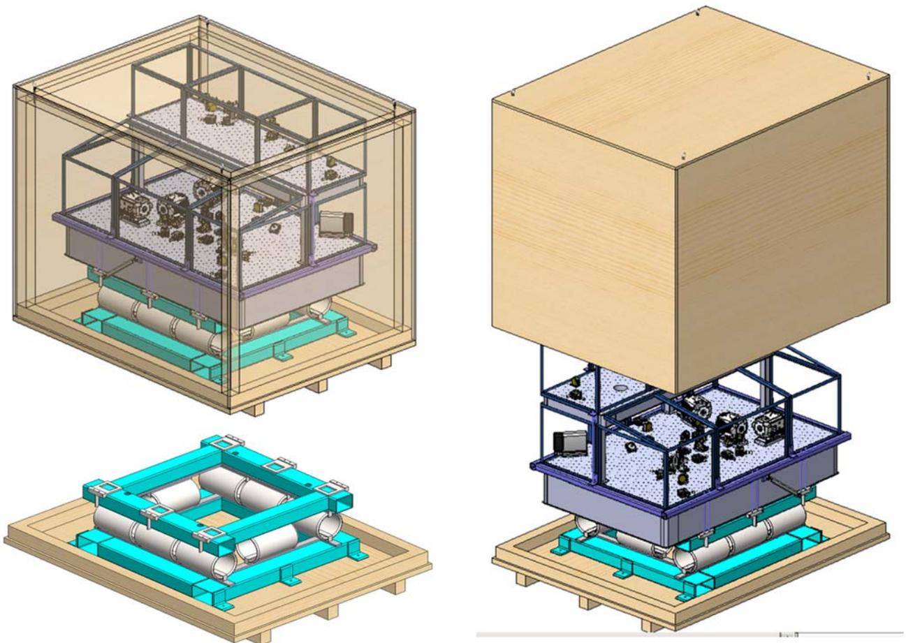
**Figure 2.4-1:** Special handling crate for the table and components. Top-left view shows the full assembly. Right-hand view shows the removal of the top of the crate to access the table. Bottom-left shows the assembly of the steel frames and wire rope isolator configuration mounted to the bottom of the crate.
