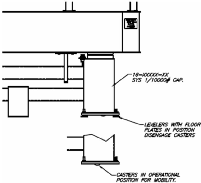
Figure 2.4-6: Table casters allow fine alignment under load.
