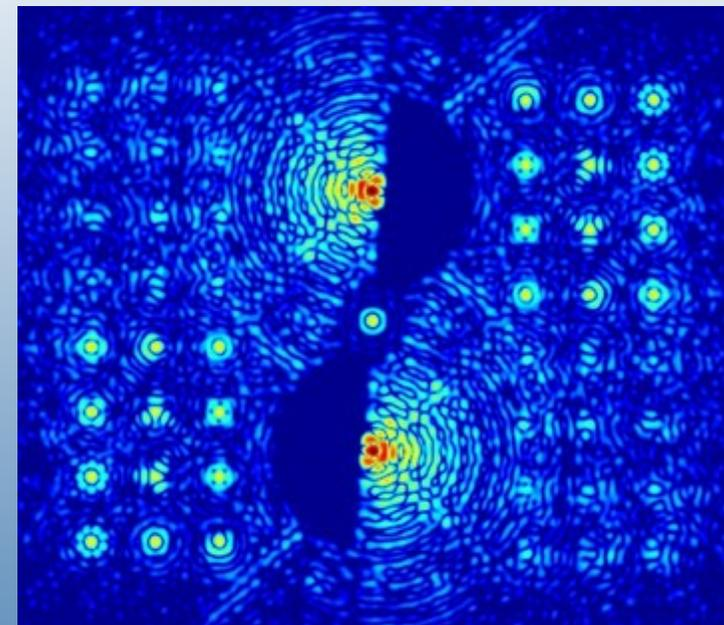
Modal WFS encoded in vAPP liquid crystal mask, brightness of spot tells amplitude of corresponding Zernike
