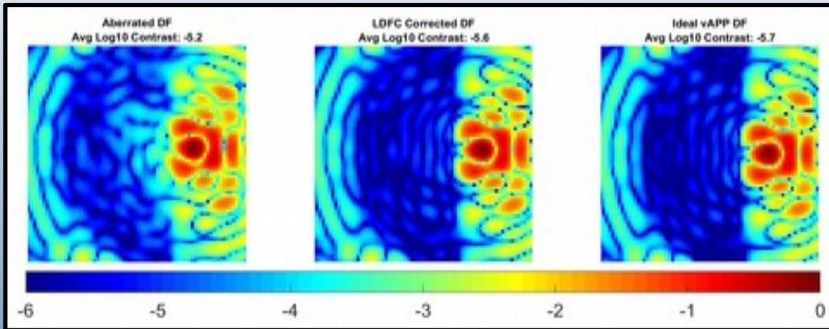
Linear Dark Field Control: using the bright field outside the dark hole to optimize contrast. Above: simulation of LDFC on a vAPP PSF.
