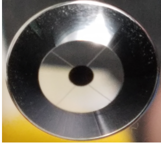
(a) Reflective Magellan pupil mask elongated along the X axis to match the incoming beam footprint at a 30^\circ angle
