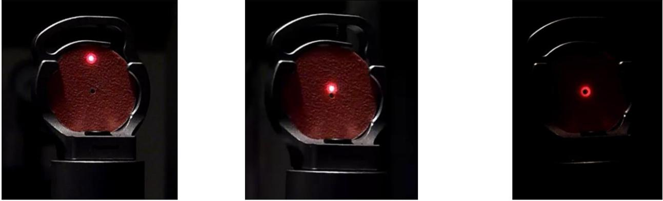
**Figure 14** – [Video 1](#) shows the first observation of the K-mirror alignment over one  $360^\circ$  rotation. The beam deviation was  $\pm 29$  arcminutes. [Video 2](#) shows an improved alignment of the K-mirror where the beam deviation was  $\pm 7$  arcminutes. The beam also starts to rotate twice around the target, an expected result when rotating a mirror. [Video 3](#) shows the final K-mirror alignment with  $\pm 1$  arcminute of wobble.
