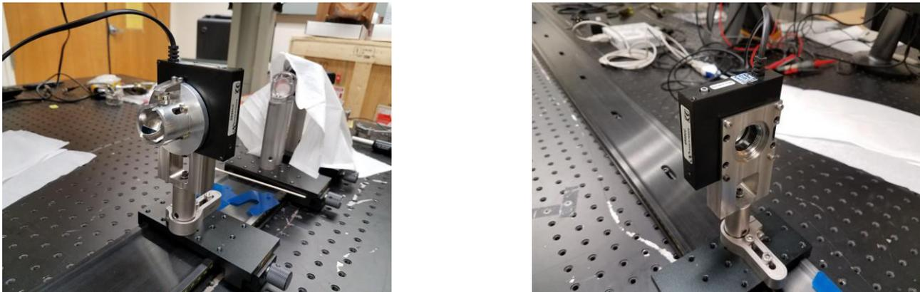
**Figure 13** – A custom stainless steel adapter was designed to mount a Polaris® 1-in diameter post to the Newport® SR50CC rotating stage. The custom mount is needed to properly bolt the rotating stage to the post and provide a more rigid structure for holding the stage.
