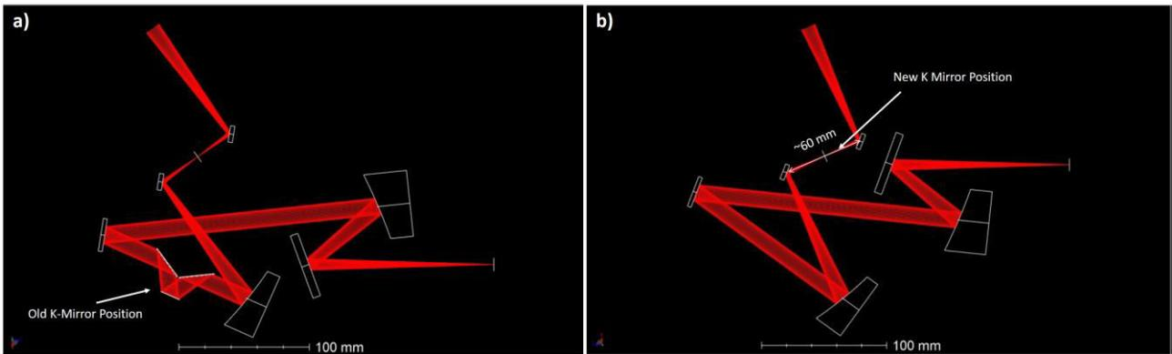
**Figure 3** – a) The initial K-Mirror position between OAPs, which created variable field curvature errors. b) New K-mirror position with correct clocking of OAPs with minimum field curvature errors. The new K-mirror position is a tight 60mm cavity where the Gregorian focus of the Magellan Clay is located. This results in the need for a compact K-Mirror design.
