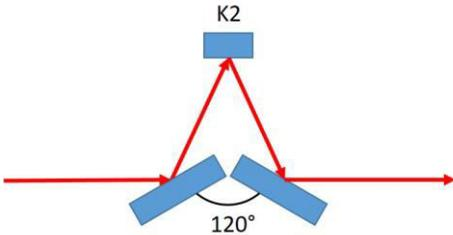
**Figure 4** – A K-Mirror consists of 3 mirrors, 2 of which are tilted by  $30^\circ$  with respect to the optical axis. The input light is coaxial with the output light
