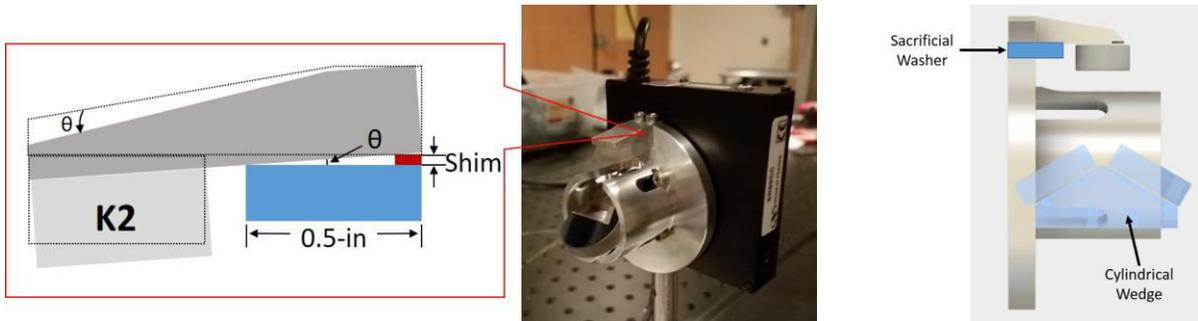
**Figure 11** – The K2 mirror may be tilted by use of shim stock (left). Placing shim stock underneath the K2 wedge allows the mirror to be tilted as needed. The K2 mirror may be shifted in piston by changing the thickness of the “sacrificial washer”—an aluminum spacer (right).
