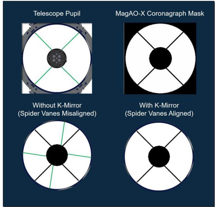
**Figure 2** – The Magellan Clay optical design produces a pupil that is asymmetric (top-left) and requires a vector Apodizing Phase Plate (vAPP)<sup>6</sup> coronagraphic mask (top-right). As the telescope rotates, the coronagraphic pupil mask is misaligned in clocking with the pupil (bottom-left). A K-mirror is therefore needed to de-rotate the pupil as the telescope tracks the sky and keep the mask aligned (bottom-right) with the pupil.
