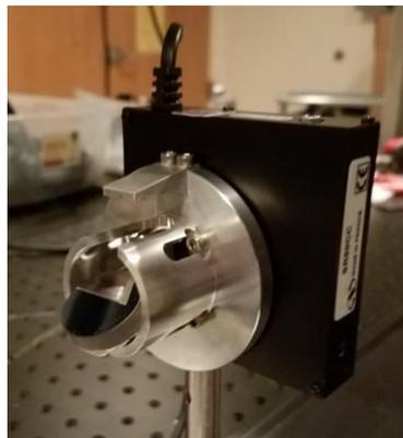
**Figure 6** – Fusion 360™ screenshot of the first K-mirror design (left). A 1-in mirror was first used for K1, while K3 is 19mm and K2 is 0.5-in. The K-mirror prototype mounted on the rotating stage (right).
