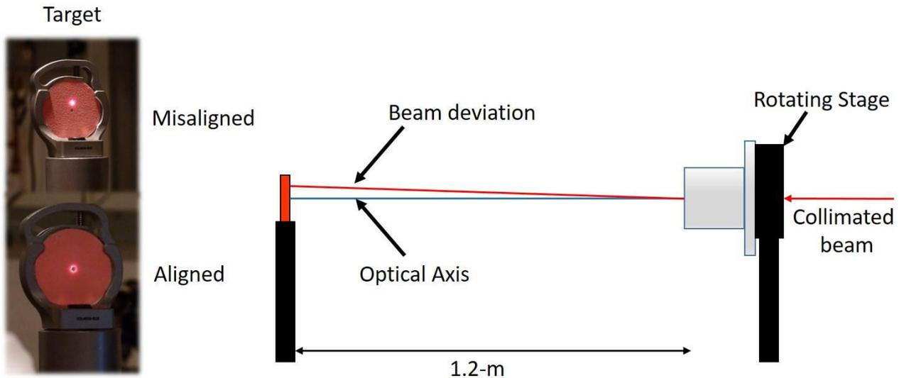
**Figure 10** - A collimated 1mm beam was set up in the lab with the K-Mirror prototype and a target mounted on a 2-meter optical rail. Using the SR50CC rotating stage, the K-Mirror was rotated and the beam offset was measured on the target. Then, K2 was adjusted to align the K-Mirror.
