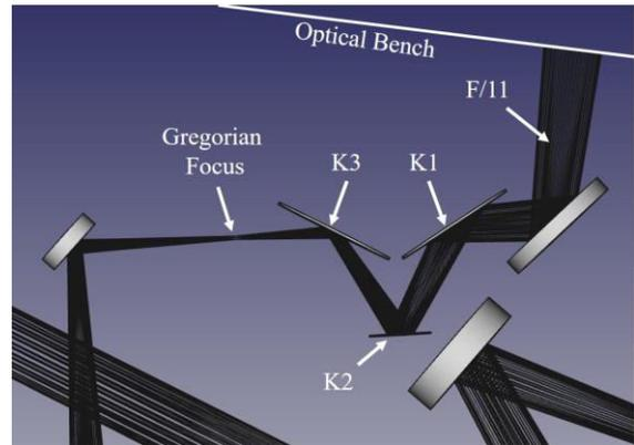
**Figure 5** – FreeCAD screenshot of the MagAO-X design. The three thin disks are the default K-mirror footprints.
