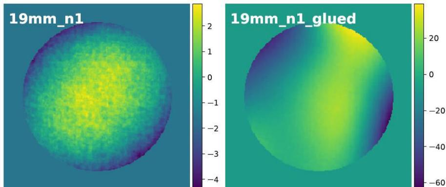
**Figure 8** – K3 before (left) and after (right) gluing. The initial measurement from the ZYGO was  $\lambda/80$  PV over the inner 80% of the surface, while after gluing, the measurement was  $\sim\lambda/8$  over 80% of the surface. However, the inner 30% (the illuminated area) is  $\sim\lambda/100$  PV. K1 and K2 have not been measured after gluing yet, but plans are to do so.
